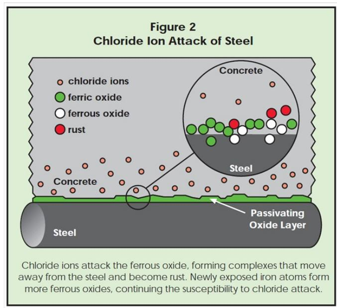
Nitrite ions assist the natural ferric oxide layer in keeping the chloride ions from complexing with ferrous ions. The nitrite does this in three ways. First, it will oxidize ferrous oxide, in order for it to become the protective ferric oxide, which is not attacked by chloride. Since the number of ferrous sites are small compared to ferric sites in the alkaline environment, essentially no nitrite is consumed (Figure 3A).
