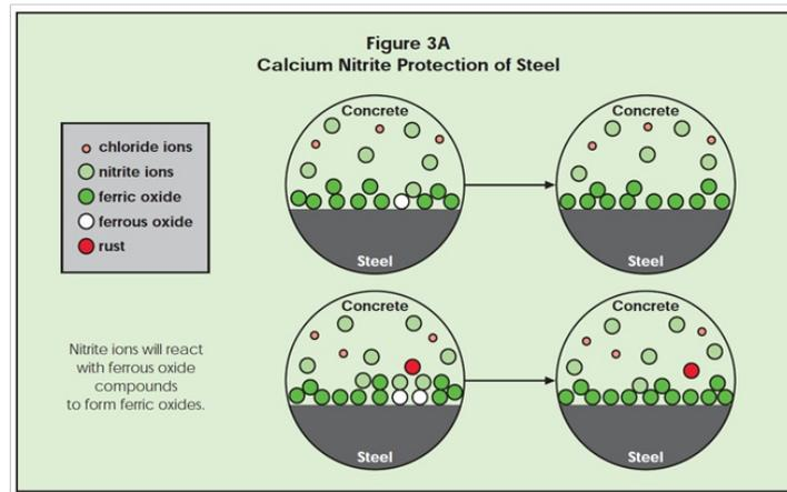
Second, the nitrite anions chemisorb at the iron surface and create a fortified ferric oxide protective layer. As in Figure 3B, the nitrite ions enhance the natural protection provided for steel by concrete. As shown in Figure 3C, ferrous oxide defects are surrounded by nitrite ions, and less likely to be exposed to chloride ion attack.
