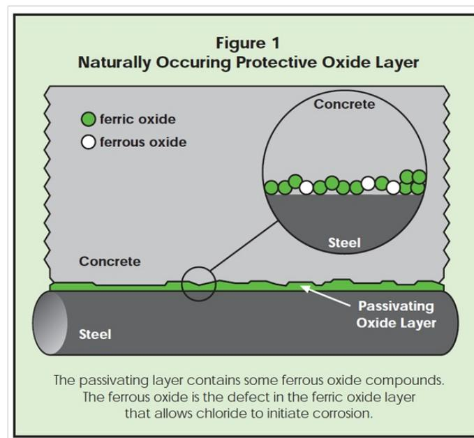
The formation of rust is an expansive reaction, creating large tensile forces inside the concrete. Staining, cracking and spalling occur in concrete containing corroding steel.
