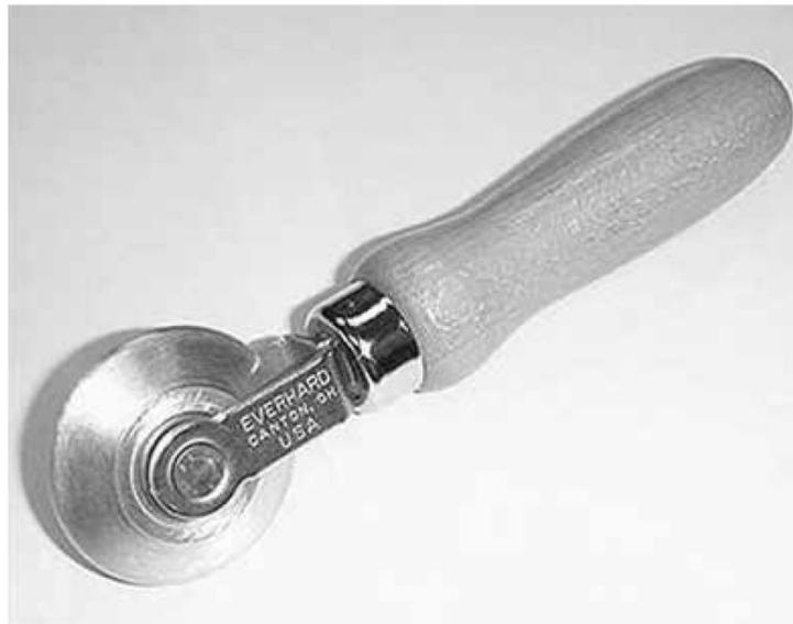
The narrow, curved, steel “Vee Roller” is rolled along this channel to conform the PREPRUFE® Tape to the step-down. Run the Vee Roller along the edges of the overlapping material that can be seen under the PREPRUFE® Tape to achieve a proper seal.
