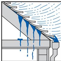
Storm-driven winds can cause sloped roof coverings to lift. Rain can then be easily driven under the roof covering directly to the unprotected roof deck where it causes leaks and damage to the interior of the structure.
