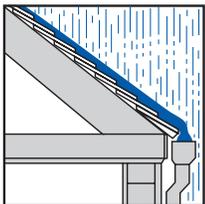
Sloped roofs are not waterproof. They protect structures by shedding rain water.
