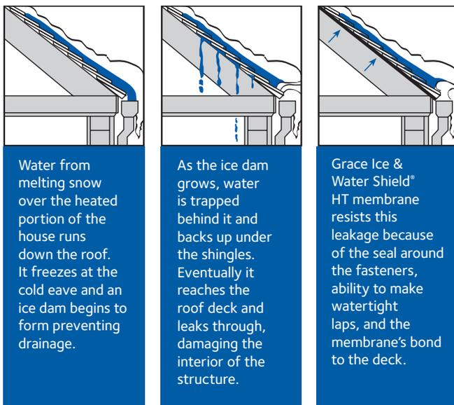
Water from melting snow over the heated portion of the house runs down the roof. It freezes at the cold eave and an ice dam begins to form preventing drainage.
