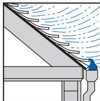
Grace Ice & Water Shield™ HT membrane applied beneath the sloped roof covering helps prevent wind-driven rain from entering the structure.
