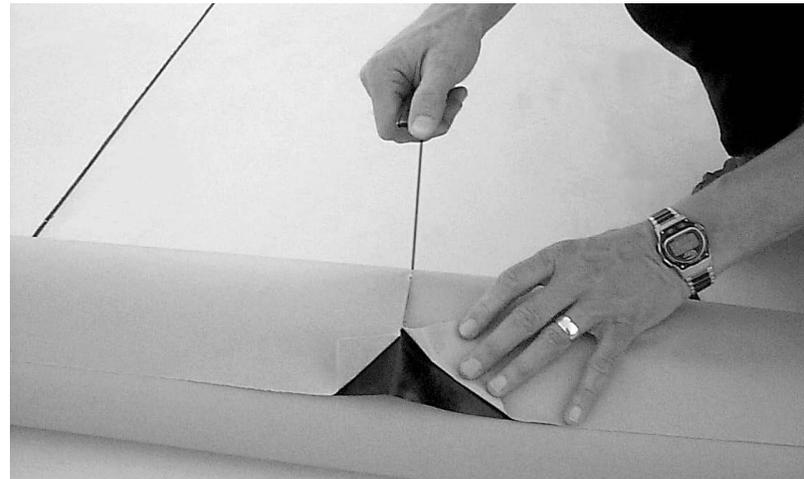
Grace Ice & Water Shield® HT roofing underlayment features the innovative Ripcord® split release on demand that is embedded between the underlayment material and the release liner. When pulled, the cord splits the release liner into two separate pieces permitting easy positioning and installation.
