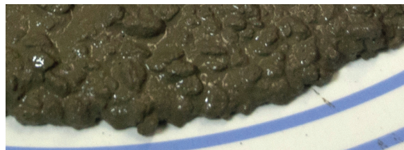
Conventional high flow concrete with CONCERA® admixtures
