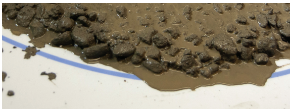
Conventional high flow concrete without CONCERA® admixtures
