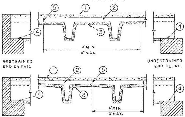
1. **Concrete Topping** — 3000 psi compressive strength. Min topping thickness, 1 in. Thickness of Spray-Applied Fire Resistive Materials Required On Flanges
