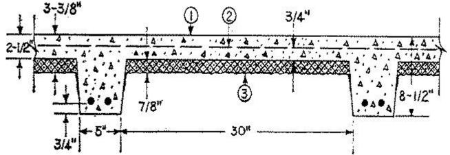
1. **Normal-Weight Concrete** — Siliceous or carbonate aggregate, 3000 psi compressive strength, to be designed with continuity over the supports.
