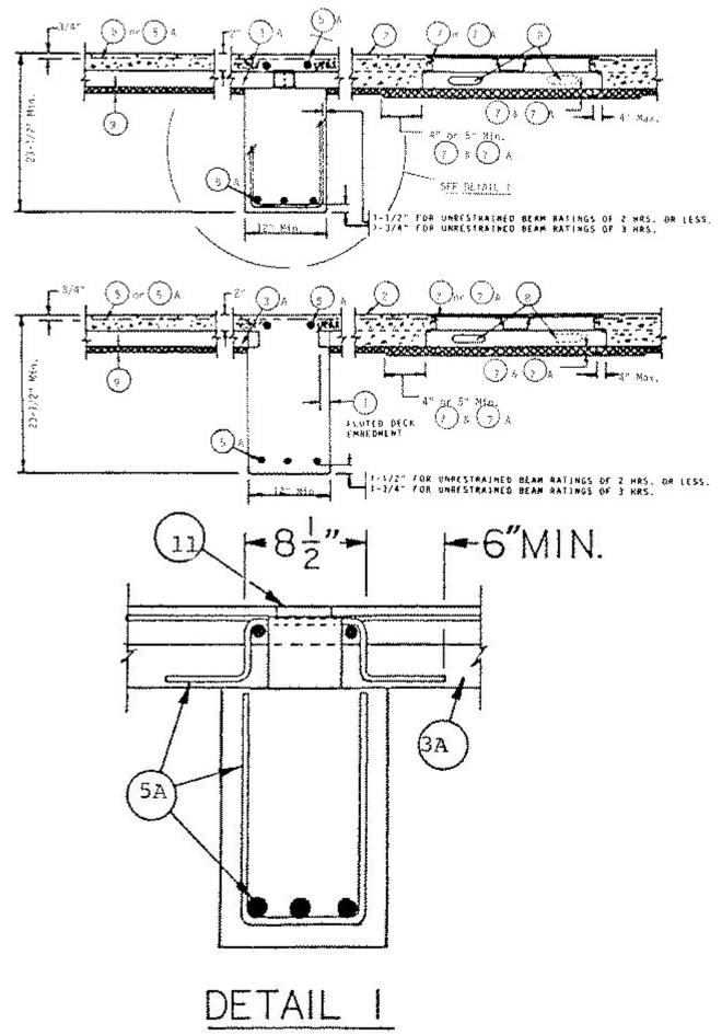
1. **Beam** — W8X20 or W8X28, min size; W8x15, min size for 1 Hr Unrestrained Beam Rating with lightweight concrete only. As an alternate to steel beams, cast in place reinforced concrete beams or girders designed in accordance with the provisions of
