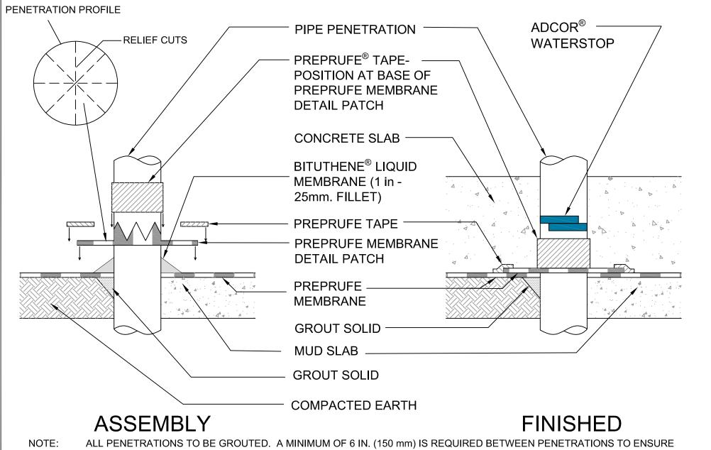
PROPER DETAILING. AVOID PLACEMENT OF MULTIPLE PENETRATIONS.
