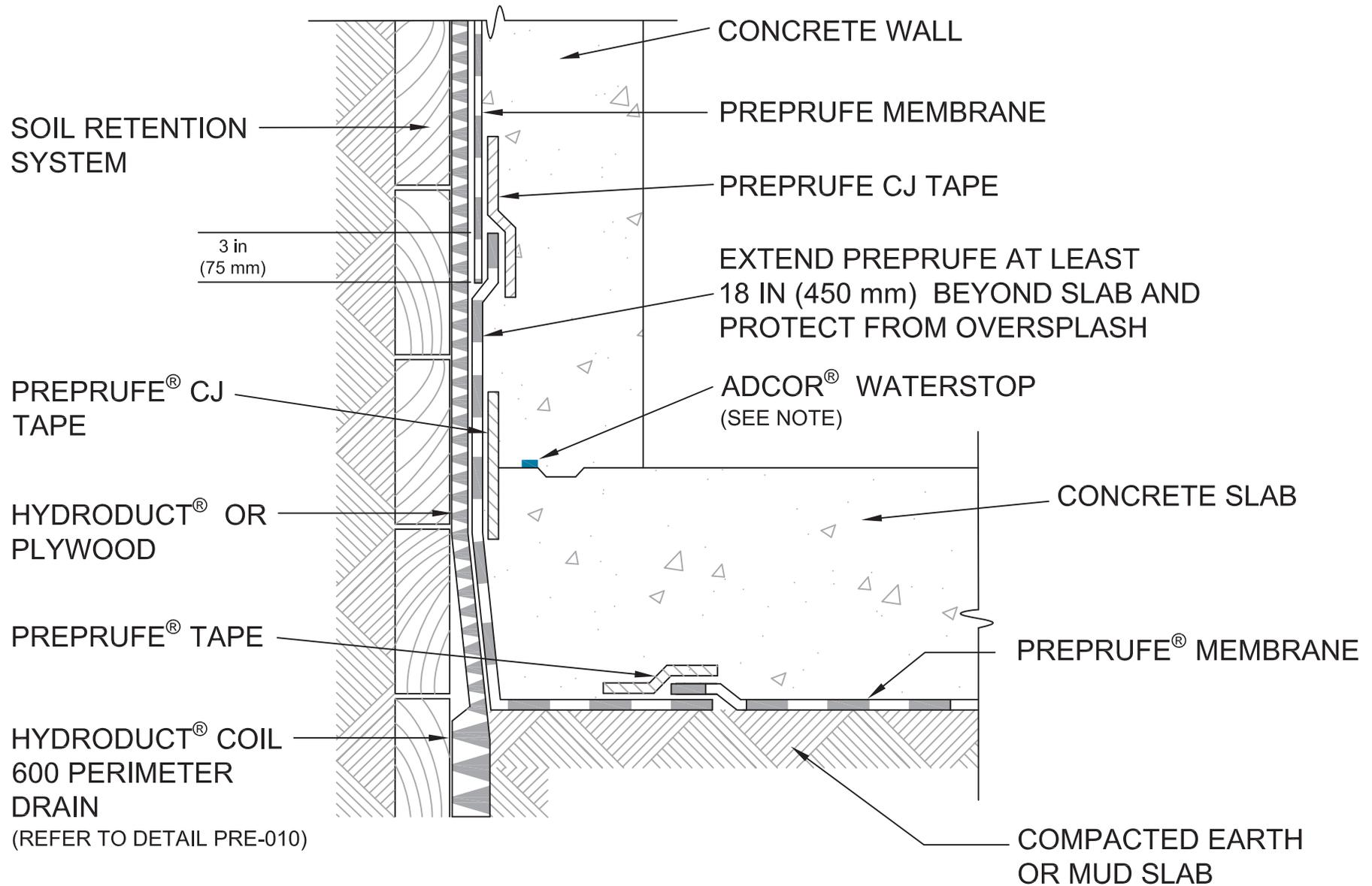
NOTE: GCP MAY REQUIRE AN ALTERNATE GCP WATERSTOP BASED ON DESIGN CONDITIONS
