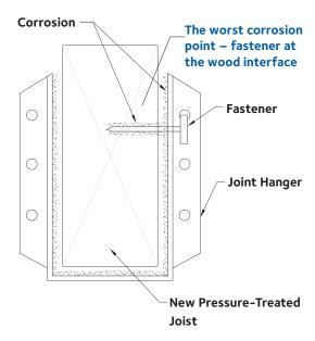
Galvanized joist hanger attached to ACQ wood, 7 months; wet conditions.
