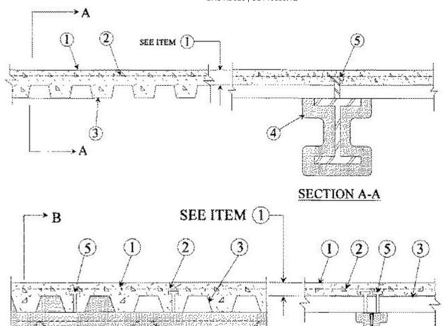
**Supports** — W8x28,W12x16 or alternate (per Section IV.6 in the front of the Fire Resistance Directory) steel beam or min 8K1 steel joists when joist substitution applied.
