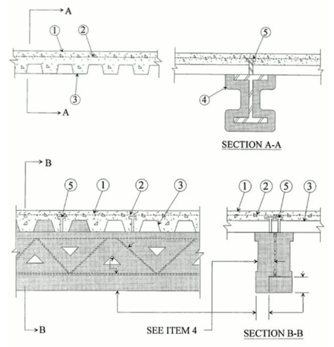
1. **Supports** — W8 x 28 or alternate (per Section IV.6 in the front of the Fire Resistance Directory) steel beam or min 10K1 steel joists when joist substitution applied.
