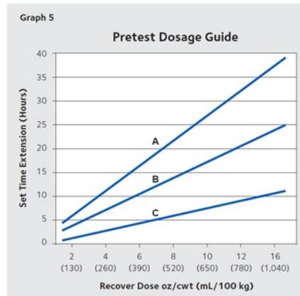
Graph 5 provides information to make initial dosage selections for pre-job testing. Lines A & B represent a typical dosage range for concrete mixtures in moderate temperature conditions.
