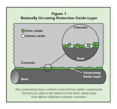
The formation of rust is an expansive reaction, creating large tensile forces inside the concrete. Staining, cracking and spalling occur in concrete containing corroding steel.
