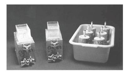
This chloride ponding test data proves that as more microsilica is added to a constant mix design, the concrete chloride permeability is reduced. These data also qualitatively agree with the AASHTO T-277 test method which states that as the coulombs measured decrease, the chloride permeability also decreases.
