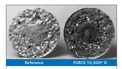
In this abrasion-erosion test, the reference disk on the left contained no microsilica. The disk on the right contained 15% microsilica (by weight of cement).
