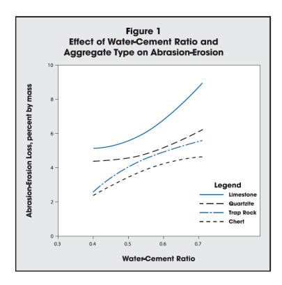
As shown, by lowering the water-cement ratio to the 0.4 - 0.5 range and using a hard aggregate like trap rock, the abrasion-erosion loss can be reduced substantially.
