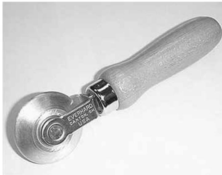
The narrow, curved, steel “Vee Roller” is rolled along this channel to conform the PREPRUFE<sup>®</sup> Tape to the step-down. Run the Vee Roller along the edges of the overlapping material that can be seen under the PREPRUFE<sup>®</sup> Tape to achieve a proper seal.
