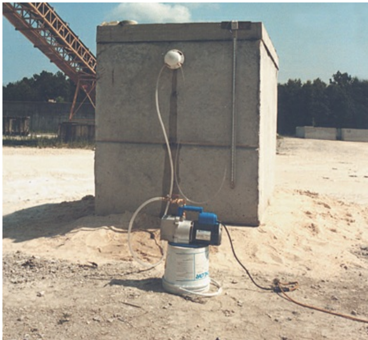
Vacuum testing of concrete septic tanks
