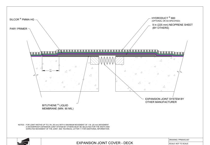
SILCOR  $^{\mbox{\scriptsize 8}}$  PMMA HG SYSTEM
