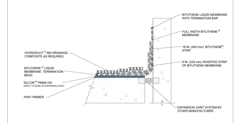
NOTES: - FOR JOINT WIDTHS UP TO 2 IN. (50 mm) WITH A MAXIMUM OF 1 IN. (25 mm) MOVEMENT. IF EXPECTED MOVEMENT IS LESS THAN 0.5 IN. (15 mm) A 6 in. (150 mm) INVERTED STRIP IS ACCEPTABLE - A WATERPROOF EXPANSION JOINT SYSTEM BY OTHERS MUST BE SELECTED FOR THE WIDTH AND EXPECTED MOVEMENT OF THE JOINT, SEE TECHNICAL LETTER 11 FOR ADDITIONAL INFORMATION.
