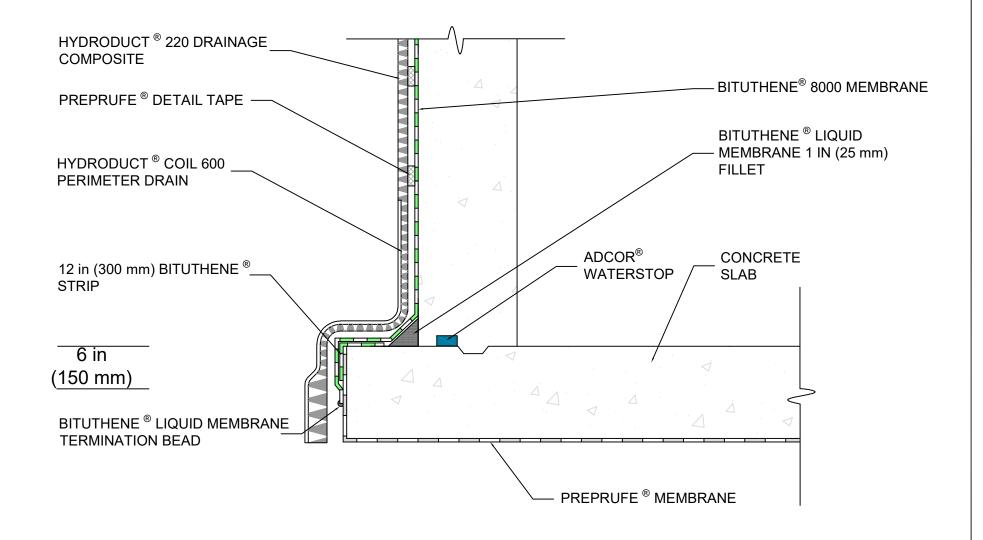
NOTE - GCP MAY REQUIRE AN ALTERNATE GCP WATERSTOP BASED ON DESIGN CONDITIONS
