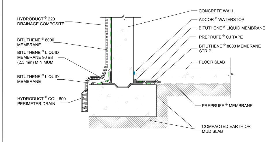
NOTES: -THE FOOTING KEYWAY SHOULD BE FORMED TO CREATE A REGULAR AND UNIFORM SHAPE ALLOWING
