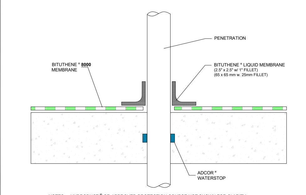
NOTES - HYDRODUCT ® OR APPROVED PROTECTION COURSE NOT SHOWN FOR CLARITY - GCP MAY REQUIRE AN ALTERNATE GCP WATERSTOP BASED ON DESIGN CONDITIONS
