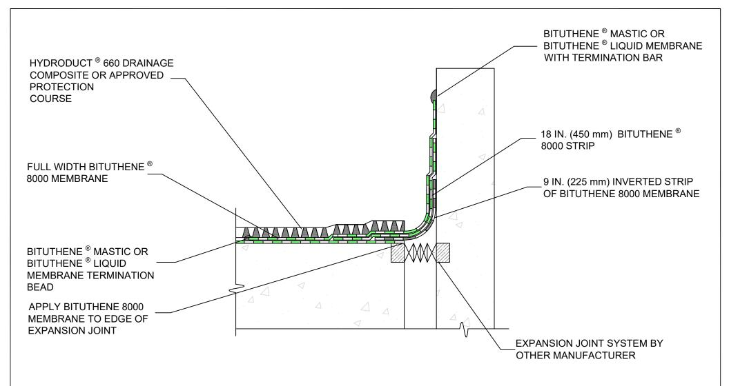
NOTES: - FOR JOINT WIDTHS UP TO 2 IN. (50 mm) WITH A MAXIMUM OF 1 IN. (25 mm) MOVEMENT. IF EXPECTED MOVEMENT IS LESS THAN 0.5 IN. (15 mm) A 6 in. (150 mm) INVERTED STRIP IS ACCEPTABLE
