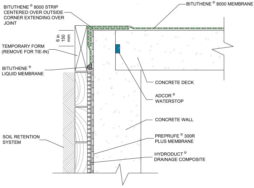
NOTE - GCP MAY REQUIRE AN ALTERNATE GCP WATERSTOP BASED ON DESIGN CONDITIONS
