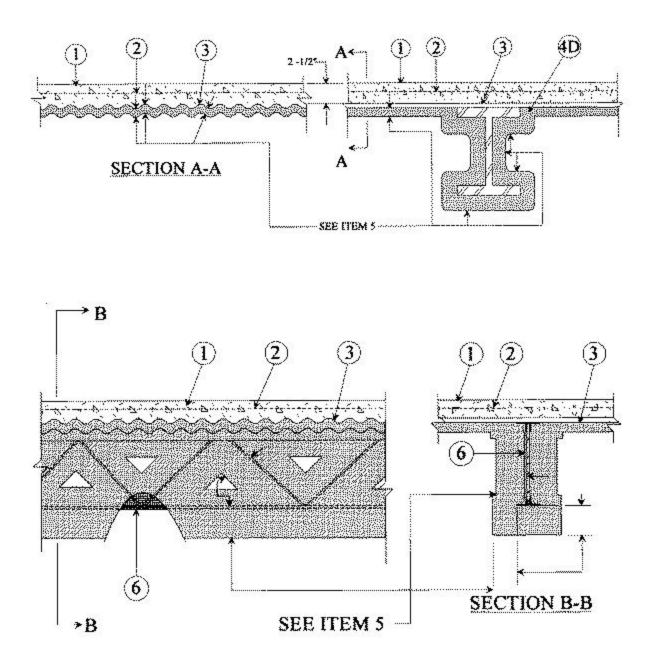
1. **Normal Weight or Lightweight Aggregate Concrete** — Normal weight carbonate or siliceous aggregate concrete, 150 plus over minus 3 pcf unit weight, 3500 psi compressive strength, vibrated. Lightweight concrete, expanded shale, clay, or slate aggregate by rotary-kiln method, 110 plus over minus 3 pcf unit weight, 3500 psi compressive strength, 4 to 7 percent entrapped air.
