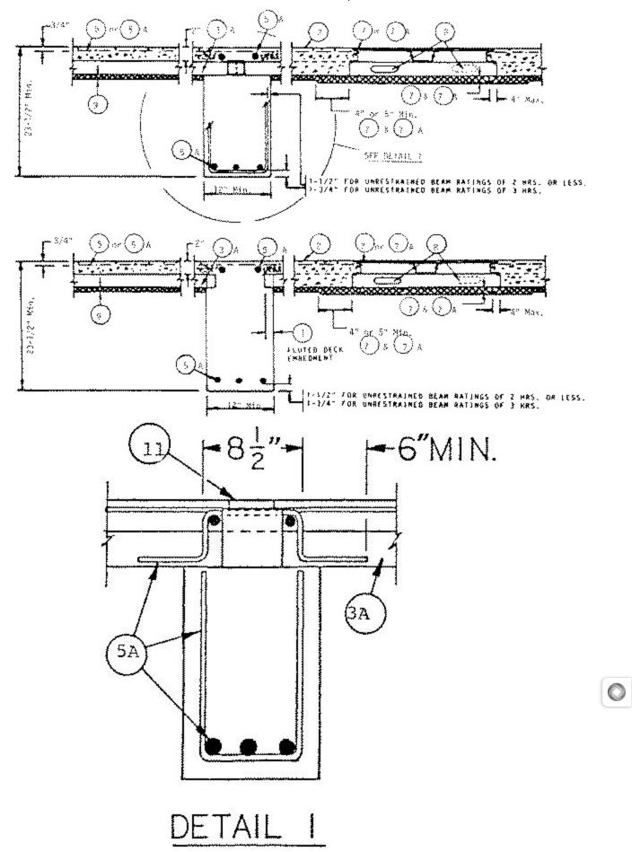
1. **Beam** — W8X20 or W8X28, min size; W8x15, min size for 1 Hr Unrestrained Beam Rating with lightweight concrete only. As an alternate to steel beams, cast in place reinforced concrete beams or girders designed in accordance with the provisions of the Building
