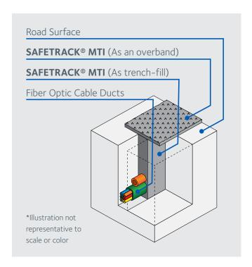
"Microtrenching" is a technique for deploying cables at a lower cost that is less invasive than usual methods.
