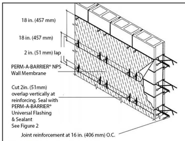
Figure 2: Horizontal Reinforcing
