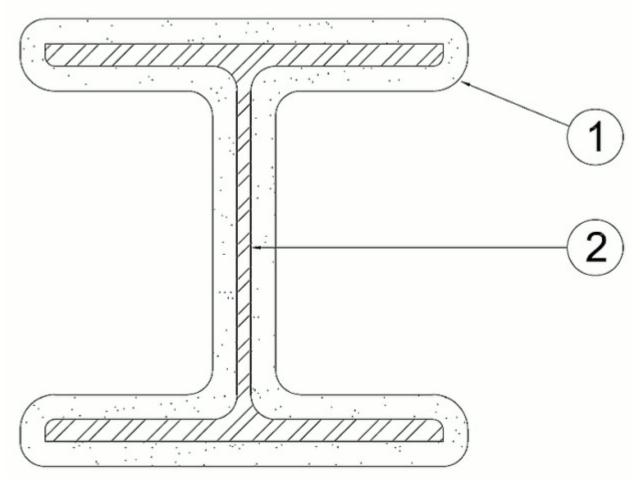
1. **Spray-Applied Resistive Material\*** — See table below for appropriate thickness. Applied in several coats to steel surfaces which must be clean and free of dirt, loose scale and oil. Min avg and min ind density of 19/18 pcf respectively for Types 7GP, 7HD, 105. Min avg and min ind density of 22/19 pcf respectively for Types KM-601, Z-106. For method of density determination refer to General Information Section.
