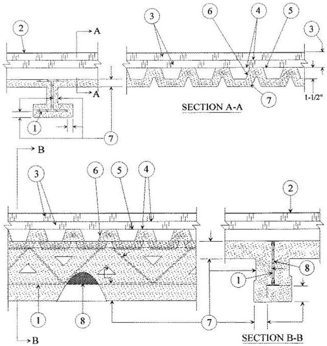
1. **Beam** — W6x16 min size or steel joist 10K1 or 16K2 min size with a max tensile stress of 30,000 psi or 12K3 min size with a max tensile stress of 24,000 psi.
