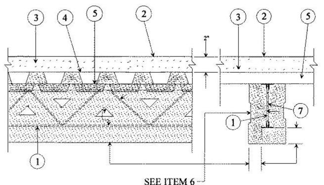
1. **Steel Joists** — 10K1 or 16K2 min size with a max tensile stress of 30,000 psi or 12K3 or 12K5 min size with a max tensile stress of 24,000 psi.
