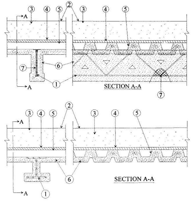
1. **Steel Supports** — W6x16 steel beam (min size) or 10K1 steel joist, (min size) having the following properties: Top chords consisting of two 1-1/4 by 1-1/4 by 0.135 in. thick steel angles; Lower chord consisting of two 1 by 1 by 0.113 in. thick steel angles; Bearing plates consisting of two 1-1/4 by 1-1/4 by 0.134 in. thick steel angles, 8 in. in length; Diagonal web members consisting of 0.561 in. diam steel rods.
