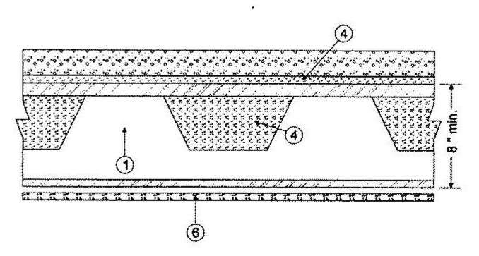
1. **Steel Beam** — Composite dissymmetric steel beam fabricated from structural steel members in accordance with the Specification for the Design, Fabrication and Erection of Structural Steel for Buildings, published by the American Institute of Steel Construction. The castellated steel beam, with a partially open web consists of the bottom flange and partial web with a bar welded to the web that serves as the top flange and conforms to the following requirements:
