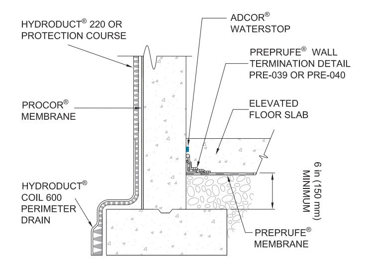
NOTES: - INTENDED FOR PROJECTS WITH PERMANENT DEWATERING OR NON- HYDROSTATIC CONDITIONS - GCP MAY REQUIRE AN ALTERNATE GCP WATERSTOP BASED ON DESIGN CONDITIONS
