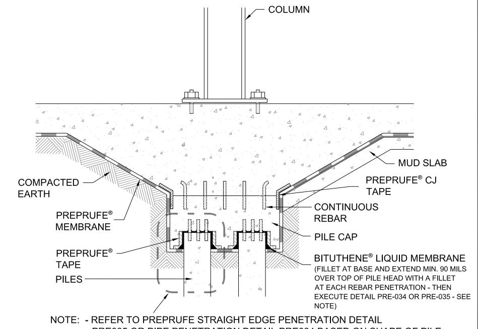
PRE035 OR PIPE PENETRATION DETAIL PRE034 BASED ON SHAPE OF PILE
