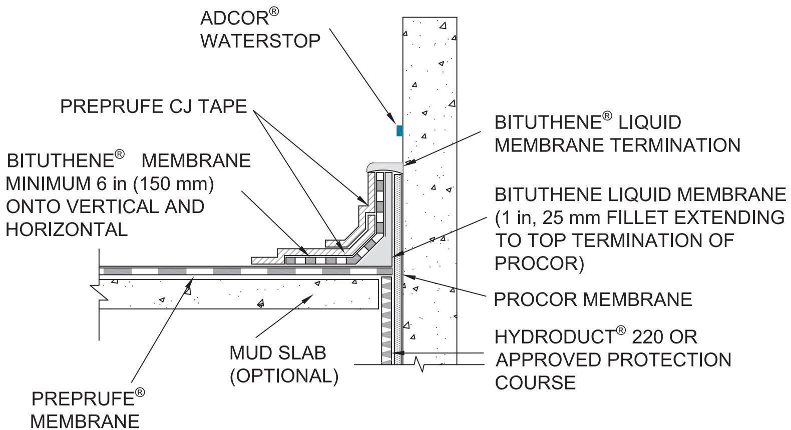
NOTES - IF A MUDSLAB IS NOT USED, THE SUBSTRATE TO ACCEPT THE BITUTHENE LIQUID MEMBRANE
