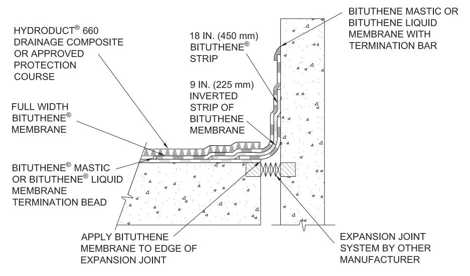
NOTES: - FOR JOINT WIDTHS UP TO 2 IN. (50 mm) WITH A MAXIMUM OF 1 IN. (25 mm) MOVEMENT. IF EXPECTED MOVEMENT IS LESS THAN 0.5 IN. (15 mm) A 6 in. (150 mm) INVERTED STRIP IS ACCEPTABLE
