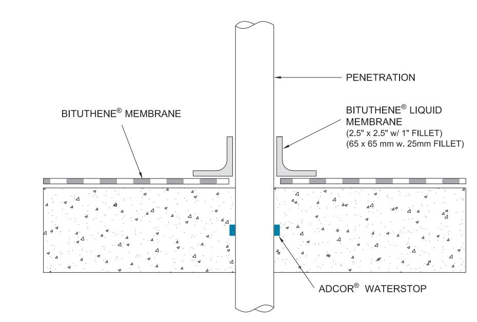
NOTES - HYDRODUCT® OR APPROVED PROTECTION COURSE NOT SHOWN FOR CLARITY - GCP MAY REQUIRE AN ALTERNATE GCP WATERSTOP BASED ON DESIGN CONDITIONS
