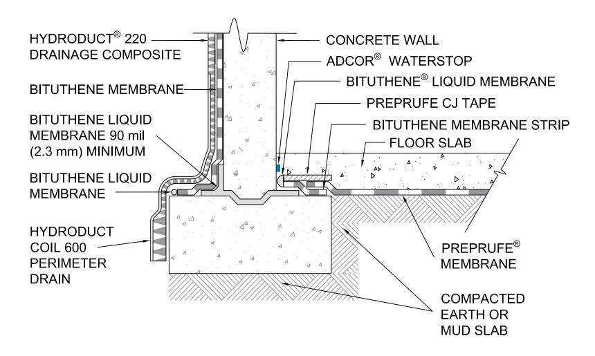
NOTES: -THE FOOTING KEYWAY SHOULD BE FORMED TO CREATE A REGULAR AND UNIFORM SHAPE ALLOWING
